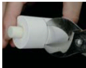
Final removal with a plaster nipper
