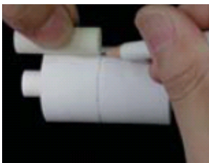
Marking the top position of the plunger
